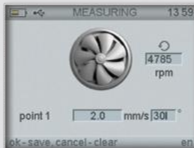
Vibration and phase measurement
