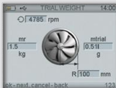
Test weight calculation and installation
